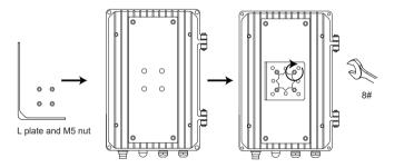
Install and fasten the repeater: lock and fix M6 nut with 10# wrench.
